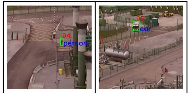
Fig. 3. Intrusion Detection at the critical infrastructure processing sequence of visible range images
