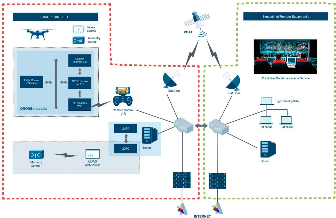
Fig. 2. NRG-5 Initial design of the Preventive Maintenance as a Service (PMaaS) for energy infrastructures
