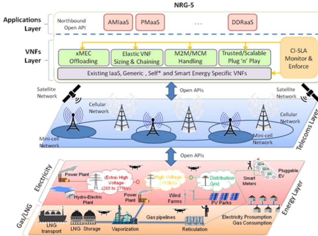
Fig. 1. NRG-5 High-level architecture
