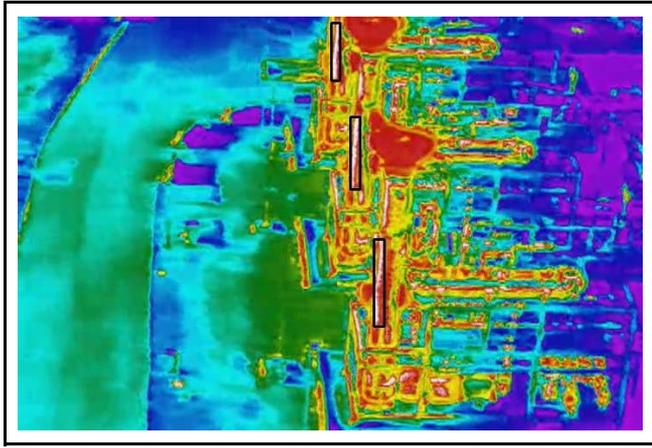
Fig. 4. Thermal image from a gas storage area in the critical infrastructure highlighting three spots where temperature is abnormally high causing an alarm to go off
